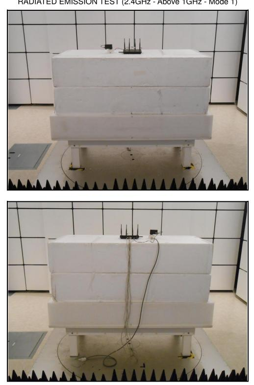
RADIATED EMISSION TEST (2.4GHz - Above 1GHz - Mode 1)
