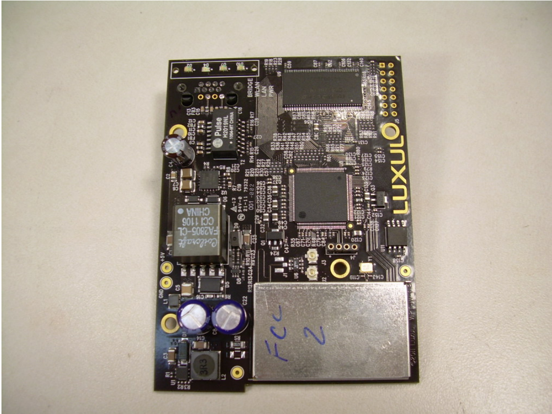
Photograph 9 – View of the Component Side of the PCB with RF Shielding in Place
