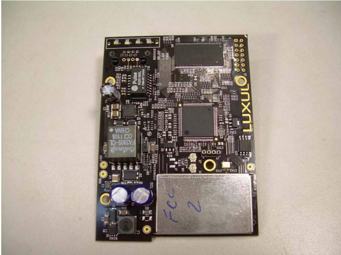
View of the Component Side of the PCB with RF Shielding in Place
