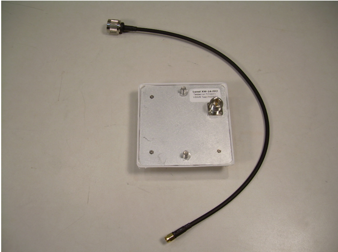
Photograph 16 – View of the Directional Antenna and Coax Cable
