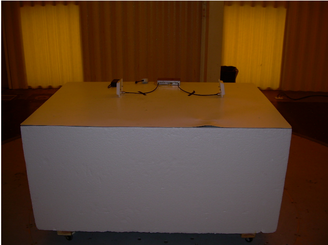
Photograph 5 – Front View Radiated Emissions Configuration – XAP-1032
