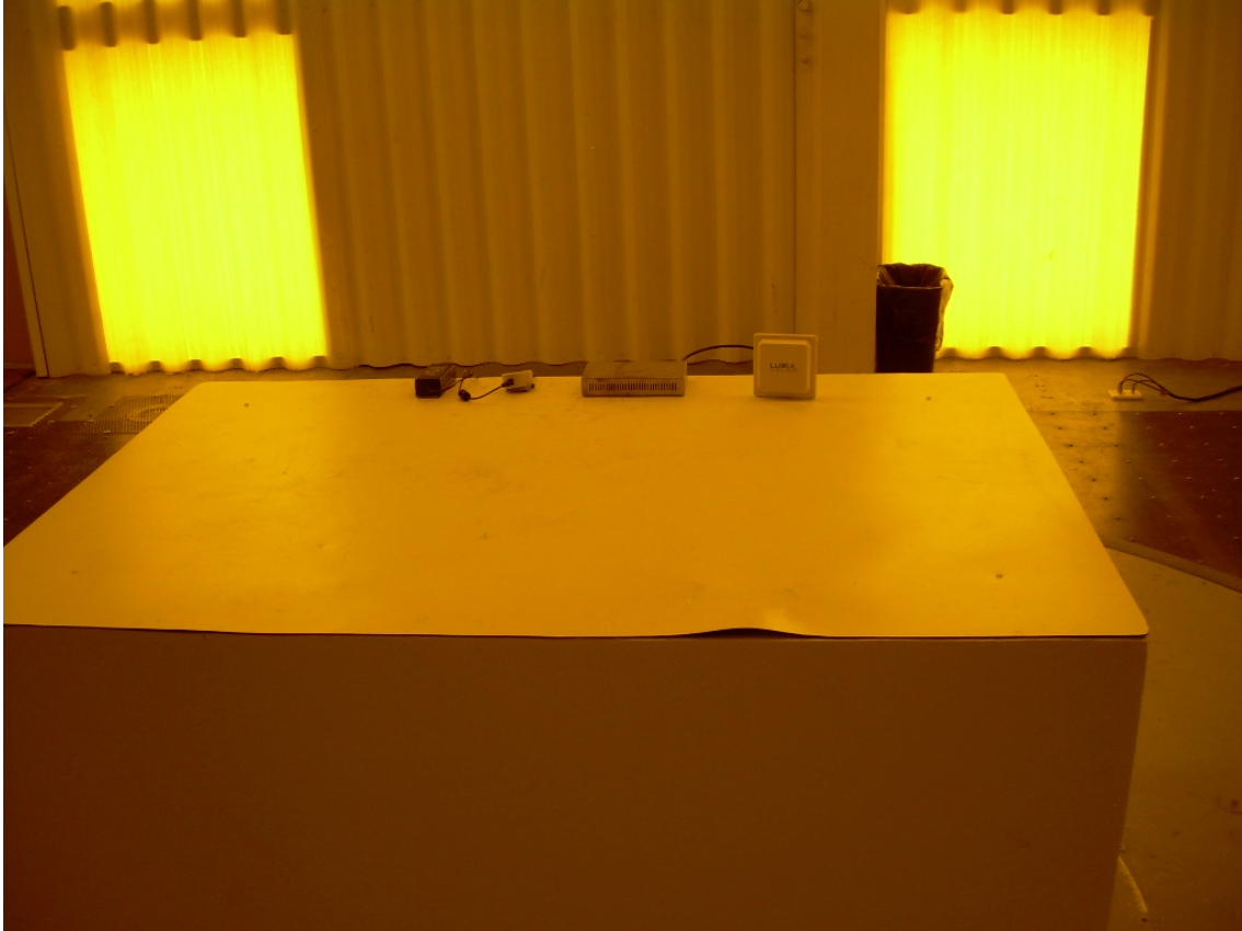
Photograph 3 – Front View Radiated Emissions Configuration – XAP-1031
