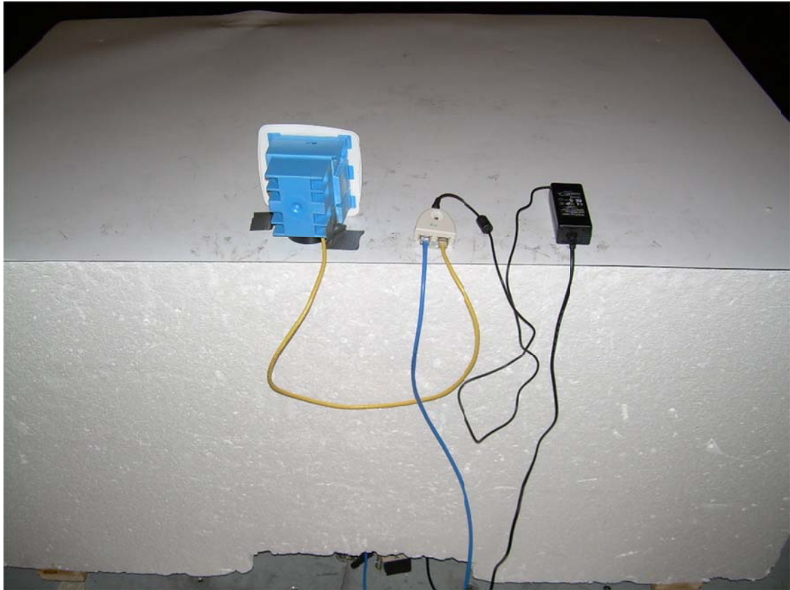
Back View Worst-Case Radiated Emissions Configuration – XAP-1010
