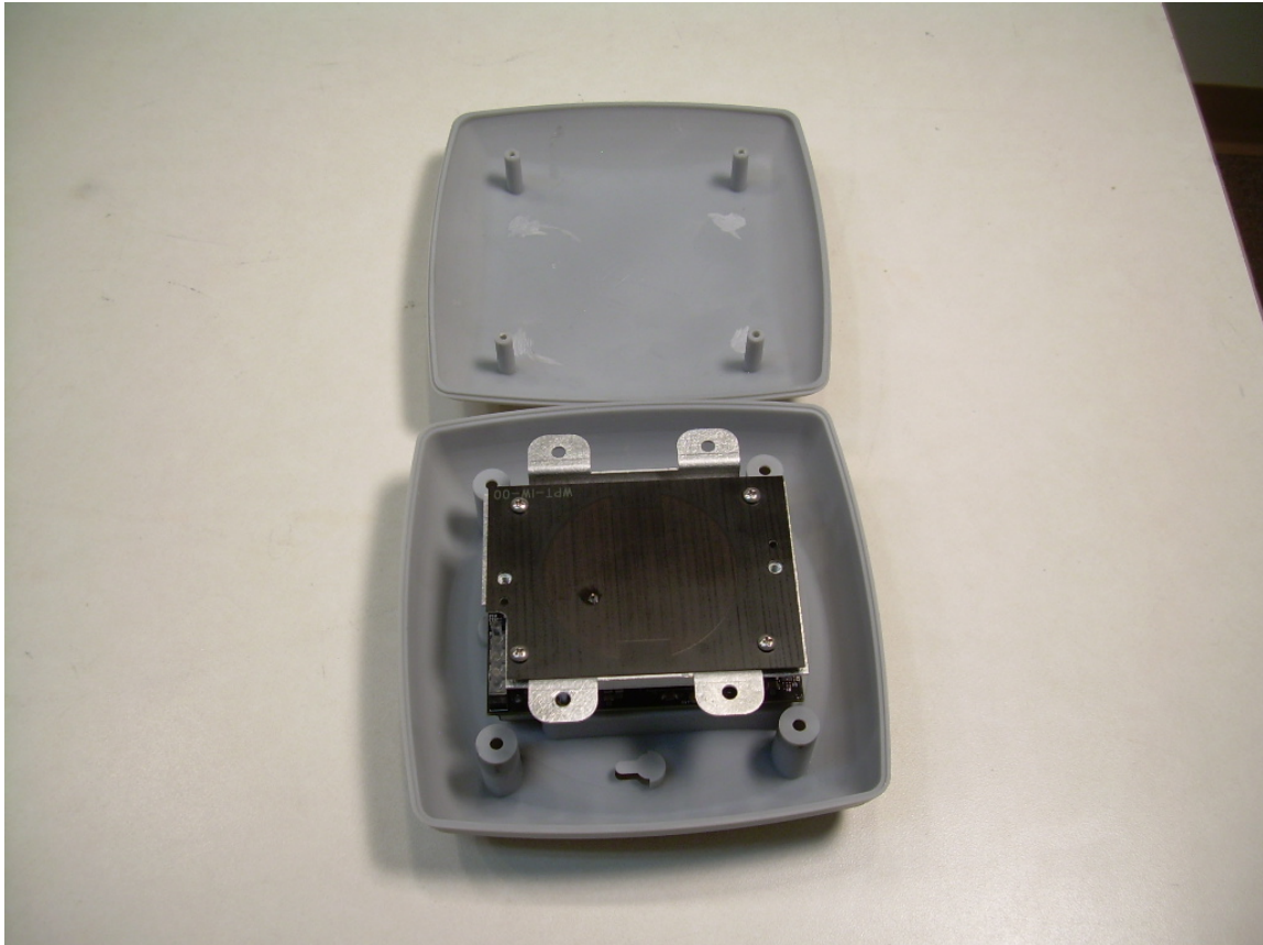
Photograph 12 – XAP-1020 Housing Open to Show Antenna and PCB Stack
