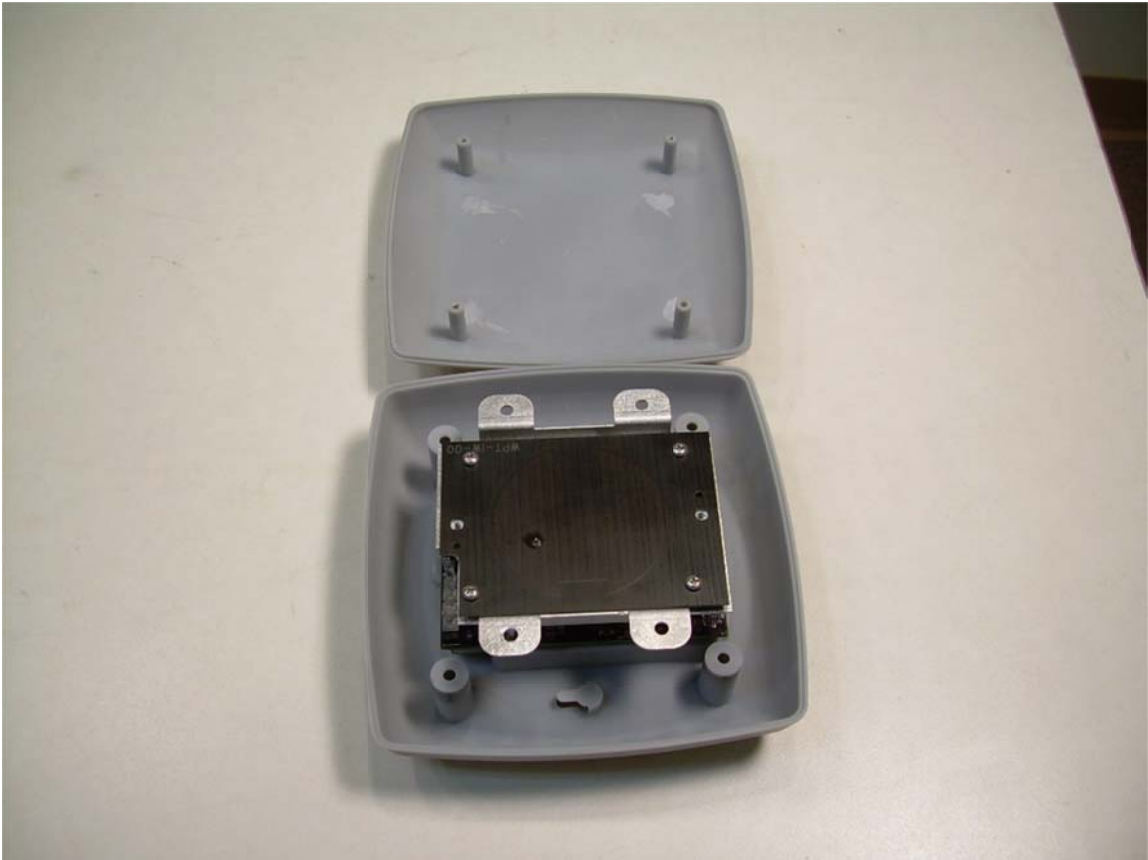
XAP-1020 Housing Open to Show Antenna and PCB Stack
