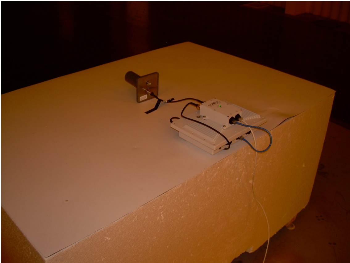
Back View of Radiated Spurious Emission Testing Set-up with Luxul XW-24-H10 Antenna
