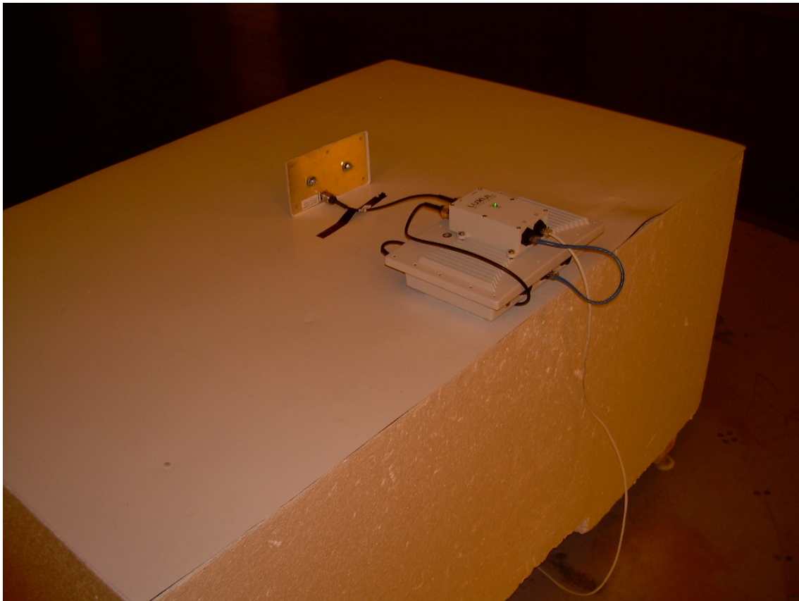
Back View of Radiated Spurious Emission Testing Set-up with Luxul XW-24-FPS11 Antenna
