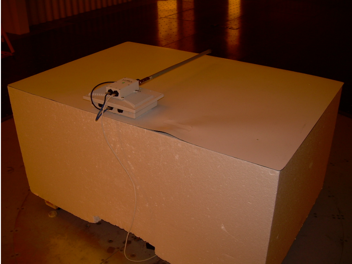
Photograph 2 - Back View Radiated Spurious Emissions Test Set-up Using the Motorola OD24M-9 Antenna
