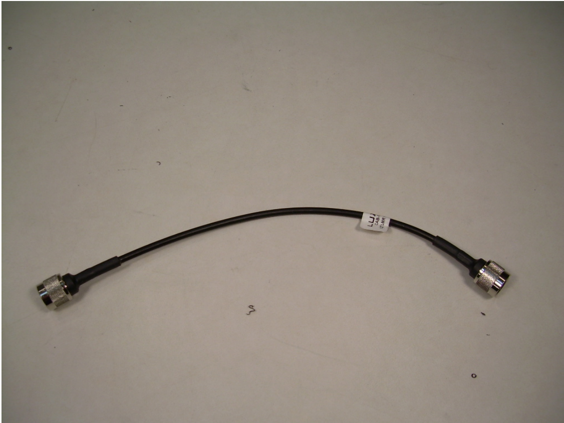
Photograph 22 - View of the 12" Coax Used from EUT to Access Point
