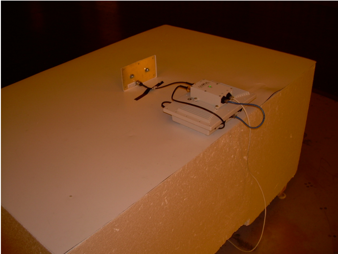
Photograph 4 - Back View of Radiated Spurious Emission Testing Set-up with Luxul XW-24-FPS11 Antenna
