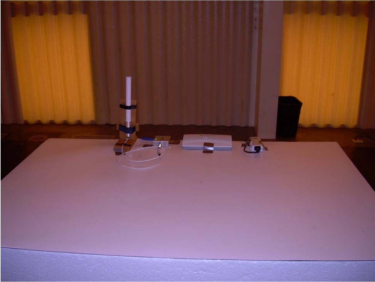
Front View Radiated Disturbance Worst Case Configuration (5 dBi Antenna)
