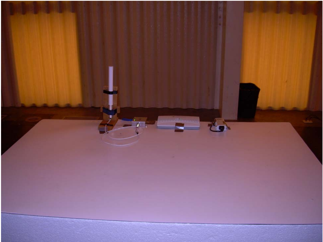
Photograph 1 - Front View Radiated Disturbance Worst Case Configuration (5 dBi Antenna)
