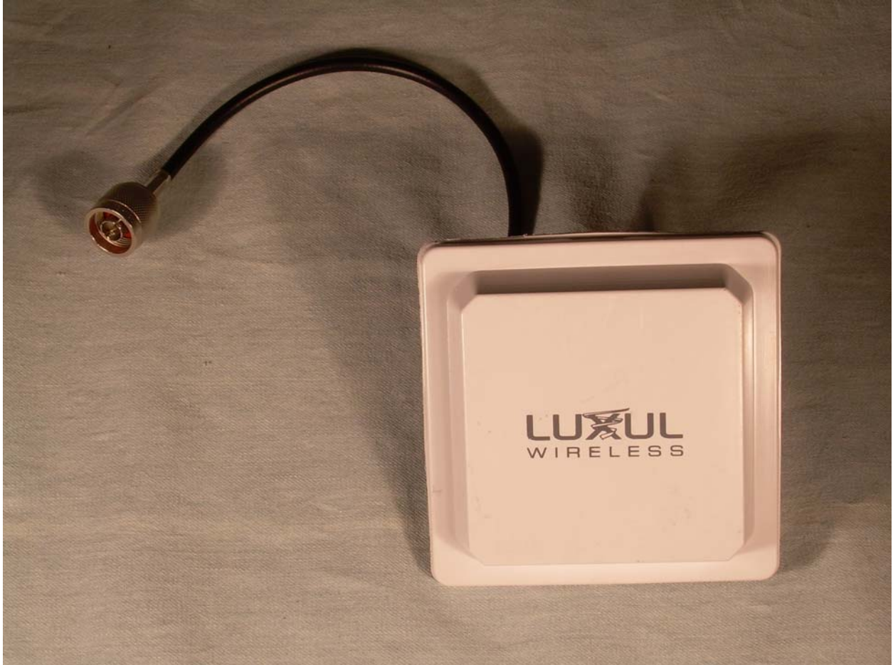
Photograph 10 - View of the 4 dBi antenna
