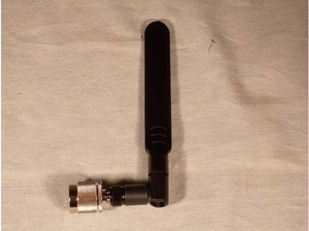
Photograph 9 - View of the 3 dBi antenna
