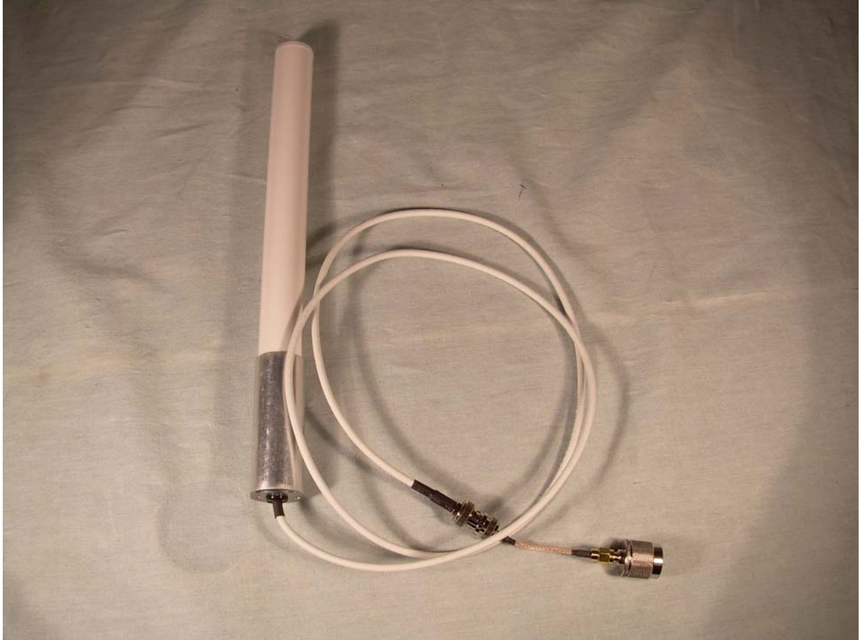
Photograph 11 - View of the 5 dBi antenna
