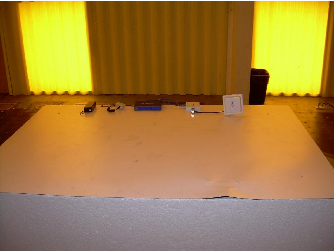
Front View Radiated Emissions Configuration Using POE Power and Single FP7 Antenna
