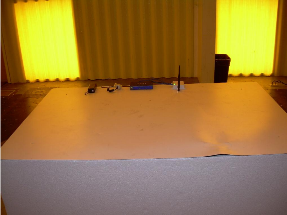
Photograph 1 – Front View Radiated Emissions Configuration Using POE Power and 5 dBi Omni Antenna
