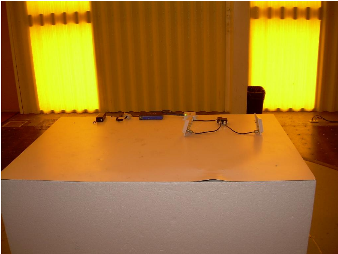
Photograph 4 – Front View Radiated Emissions Configuration Using POE Power and Dual FP7 Antennas
