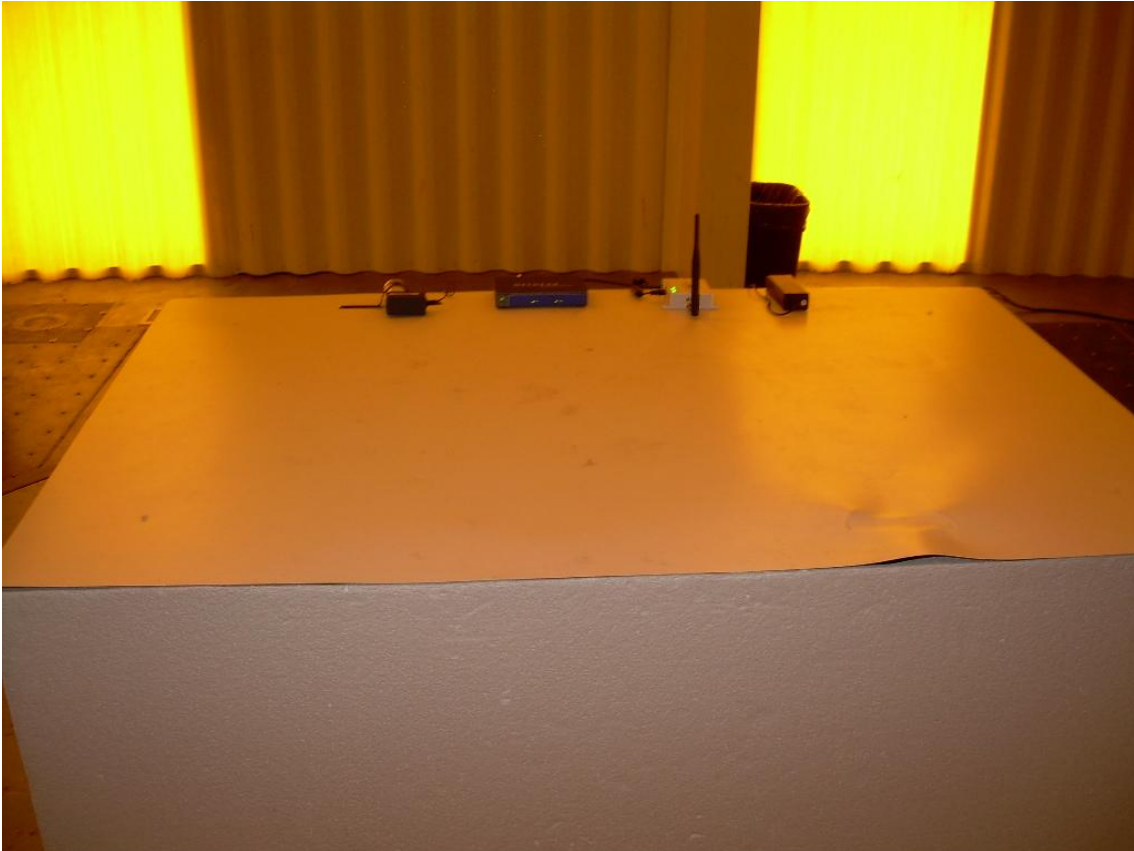
Photograph 5 – Front View Radiated Emissions Configuration Using External Power to the Access Point and 5 dBi Omni Antenna
