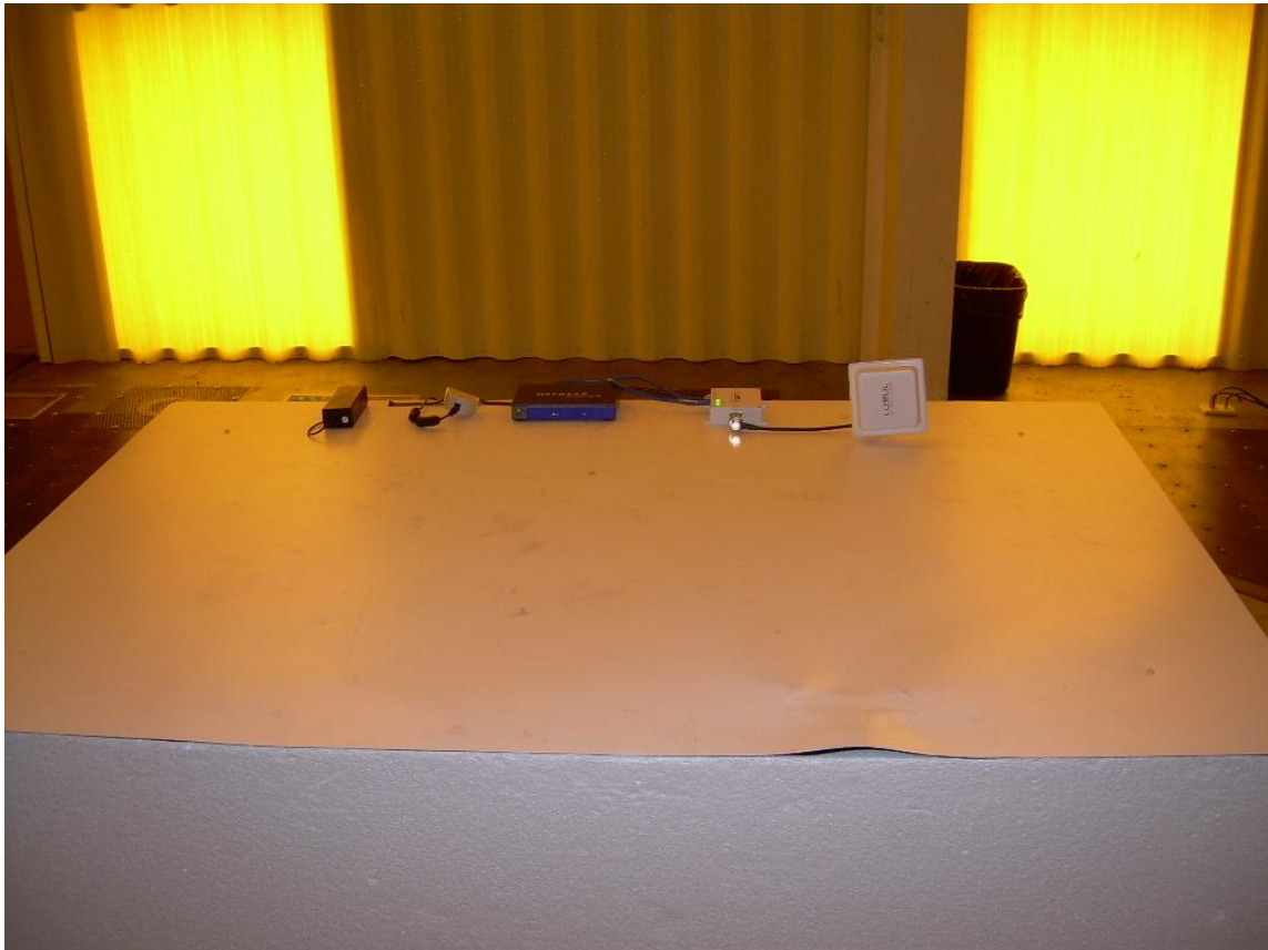
Photograph 3 – Front View Radiated Emissions Configuration Using POE Power and Single FP7 Antenna
