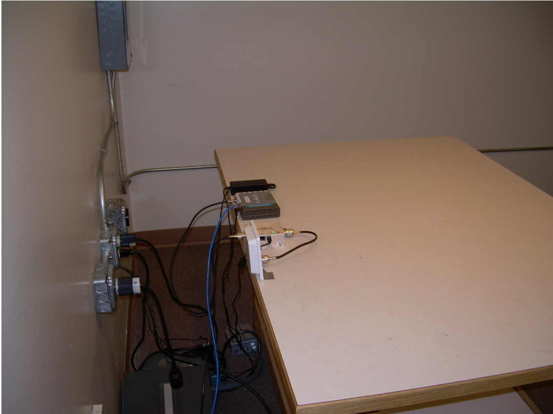
Back View Conducted Emissions Worst Case Configuration
