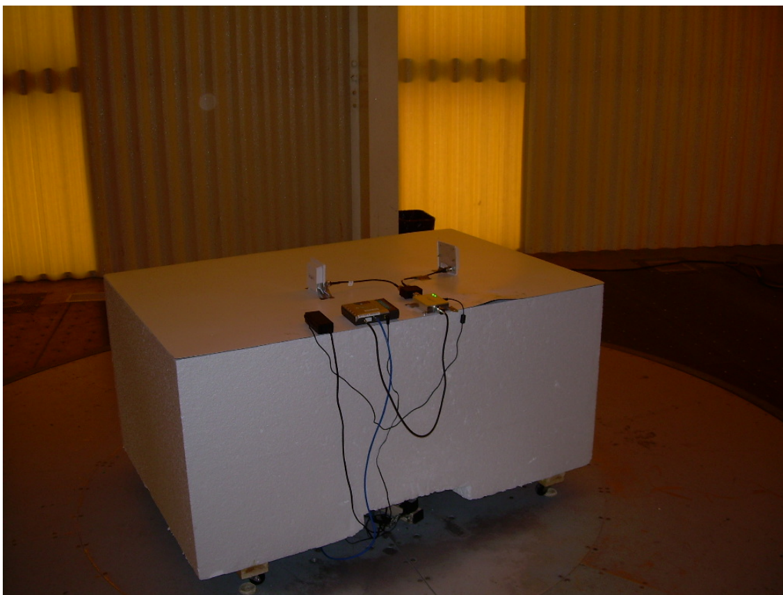
Back View of Radiated Spurious Emission Testing with Dual Antenna Configuration
