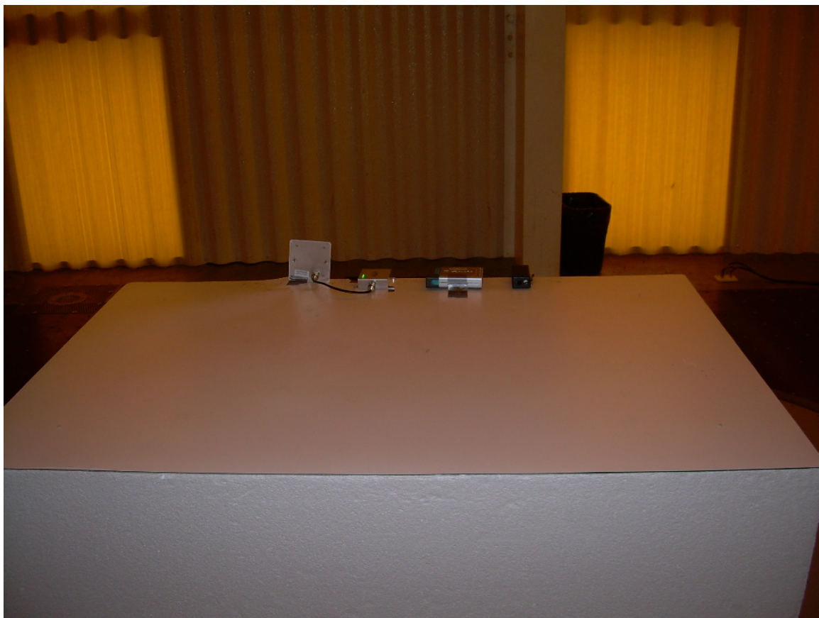
Front View Radiated Spurious Emissions Worst Case Configuration
