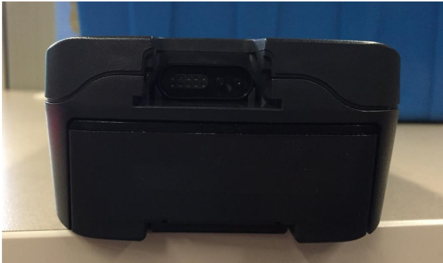
End View – Patient connector side without battery
