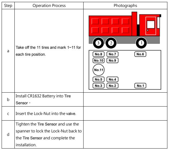
\*This product is recommended with metal valve or replace the original valve regularly to ensure better quality.
