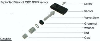
Each time a tire is serviced or dismounted, or if the sensor is removed or replaced , it is MANDATORY to replace the grommet, washer, nut, and valve core to ensure proper sealing.
