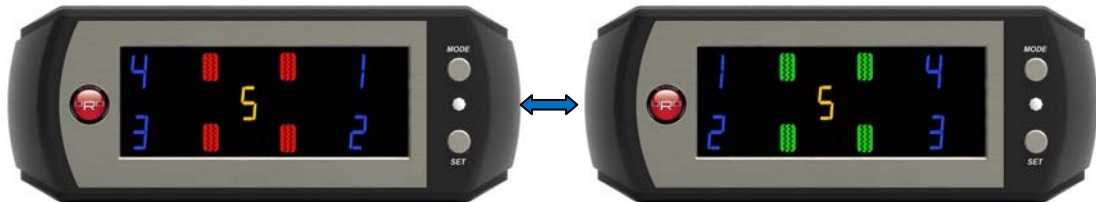
Mode 5: Right Side and Left Side Tire Parallel Exchange
