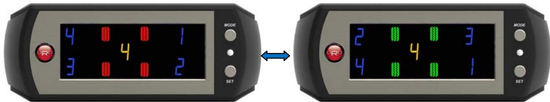
Mode 4: Rear Tire Diagonal Exchange, Front Tire Parallel Exchange to Rear
