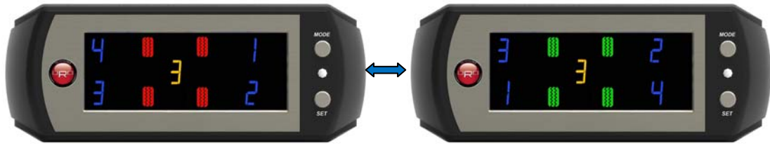
Mode 4: Rear Tire Diagonal Exchange, Front Tire Parallel Exchange to Rear
