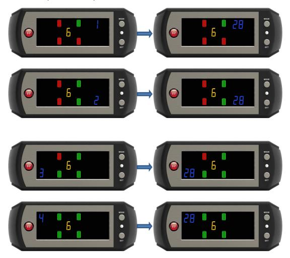
a. Depress the **SET** key to skip LF relearn or after completing the rapid deflation of Left Front tire for relearn process. The system will return to the normal operation system automatically.
