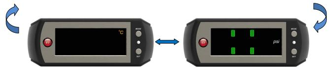
Rotate Displaying Pressure & Temperature
