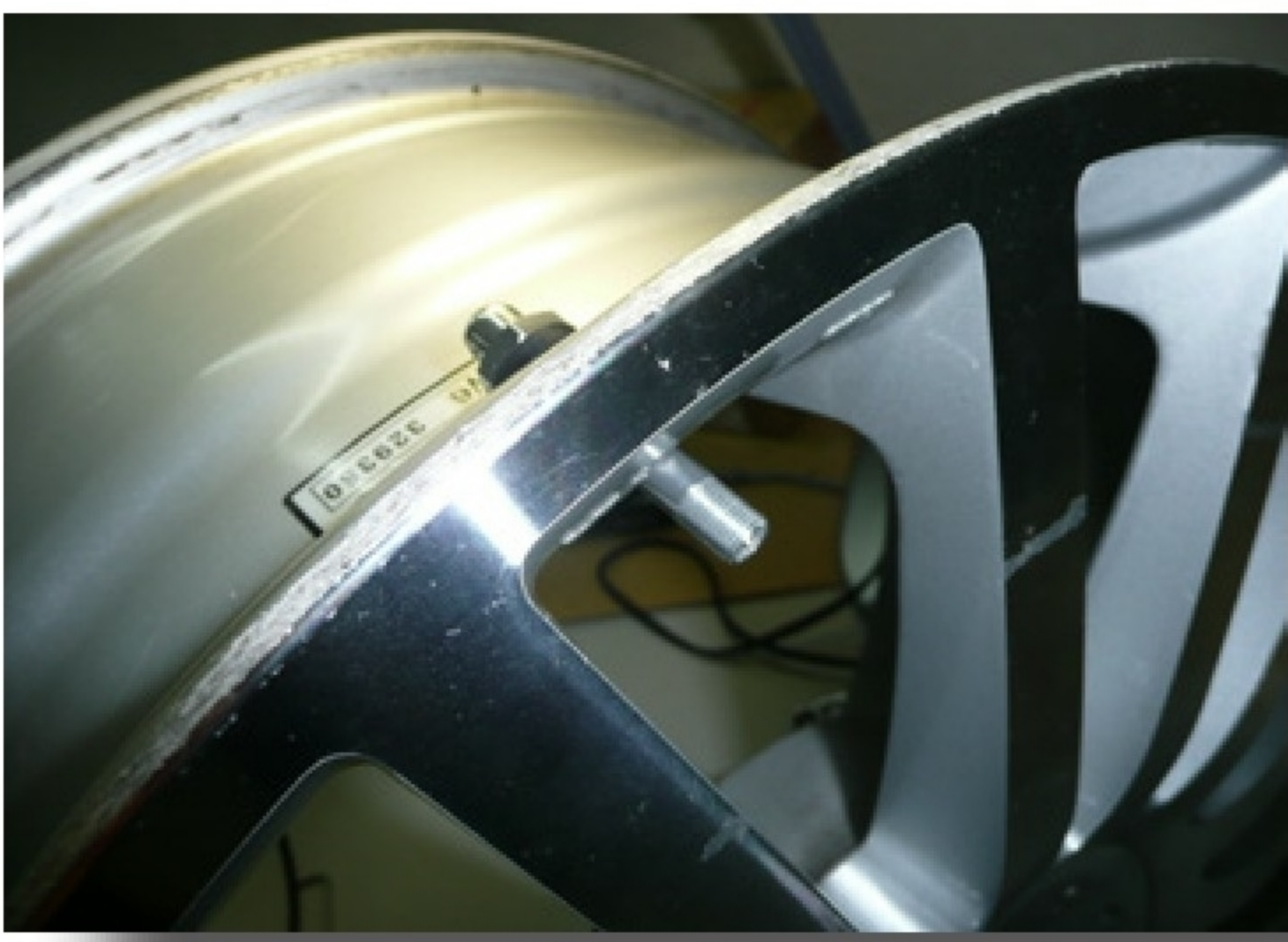
Install valve stem into the valve hole of the wheel
