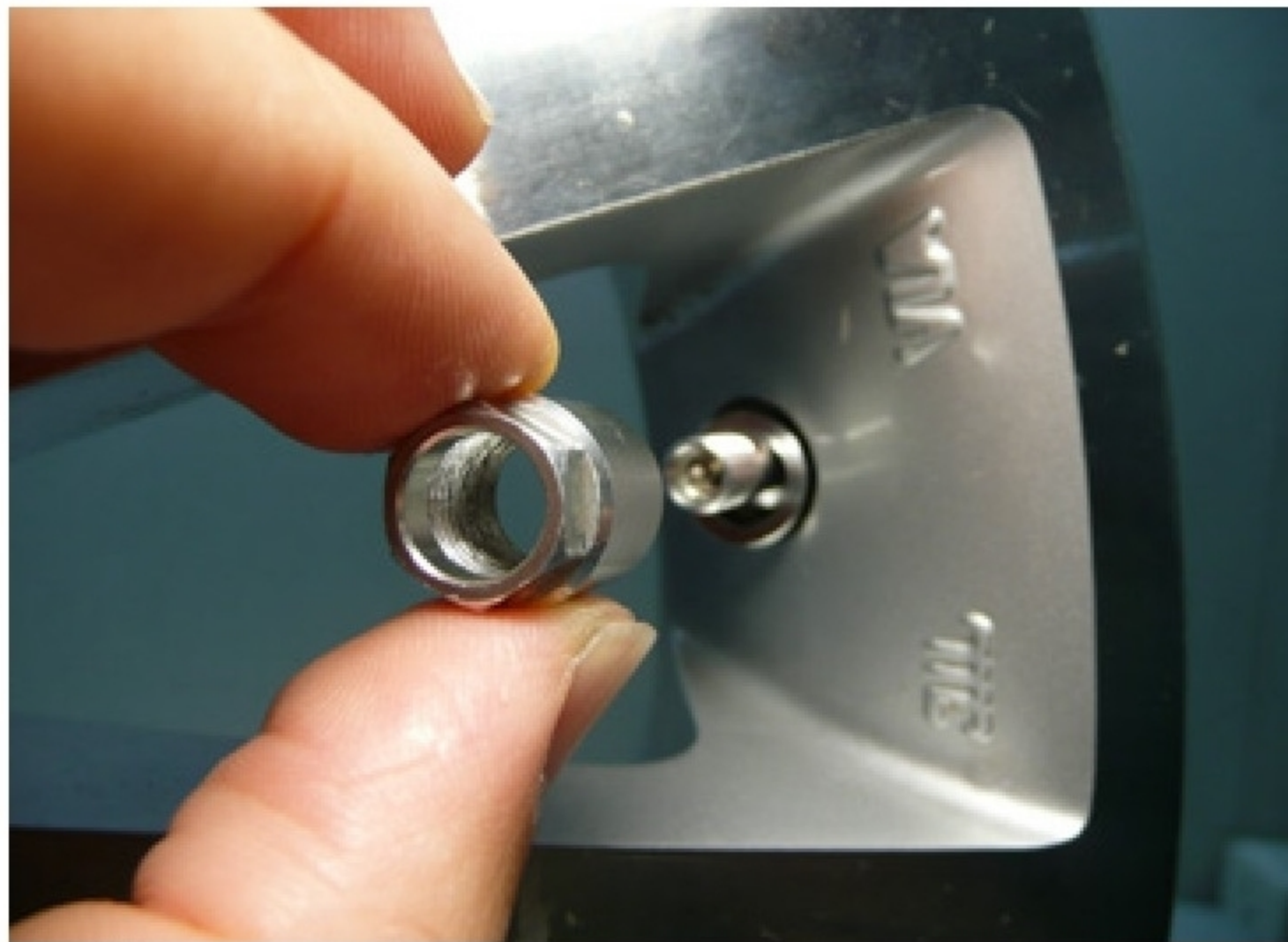
Install hexagonal nut into valve stem. Tighten the nut
