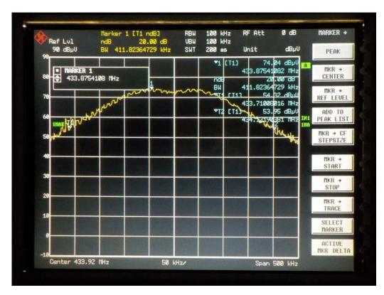
Explanation: The bandwidth fulfills the requirements of FCC § 15.231, see attached diagrams.
