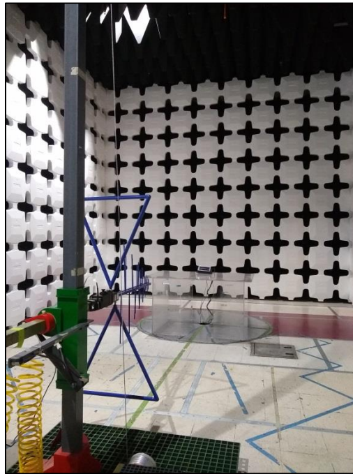
Photograph 1. Radiated Emissions, 30 MHz – 1 GHz, Test Setup
