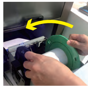
Step3. Hold onto the flange and roll it as the arrow indicated to roll out jammed paper.*
