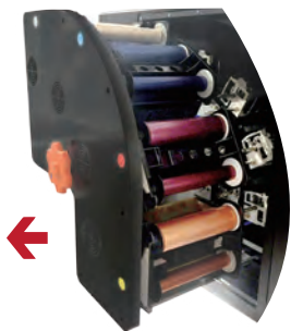
Step1. Turn off printer, open and pull out ribbon door. Make sure to separate ribbon cartridge from the printer, if ribbon is jammed into the printer, please cut it loose. *
