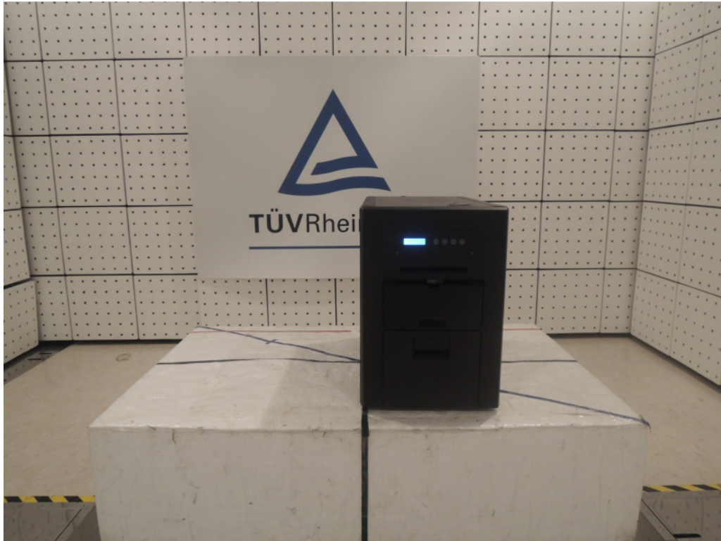
Photograph 2: Set-up for Spurious Emissions (Back View 1)
