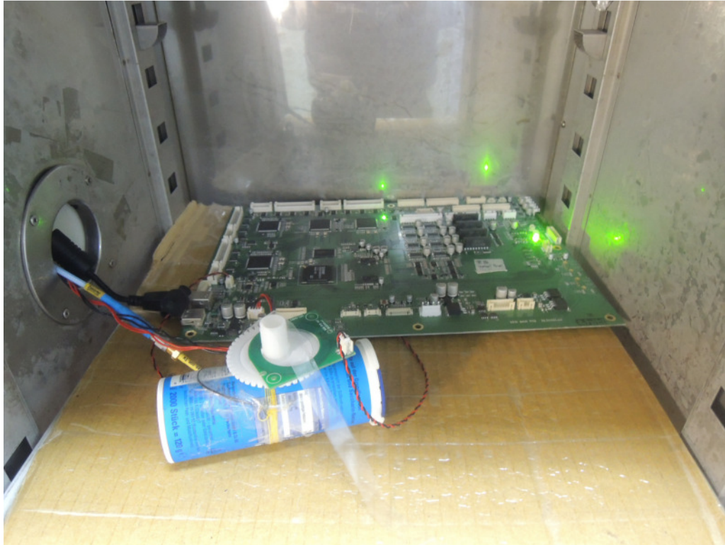
Photograph 5: Set-up for Conducted testing
