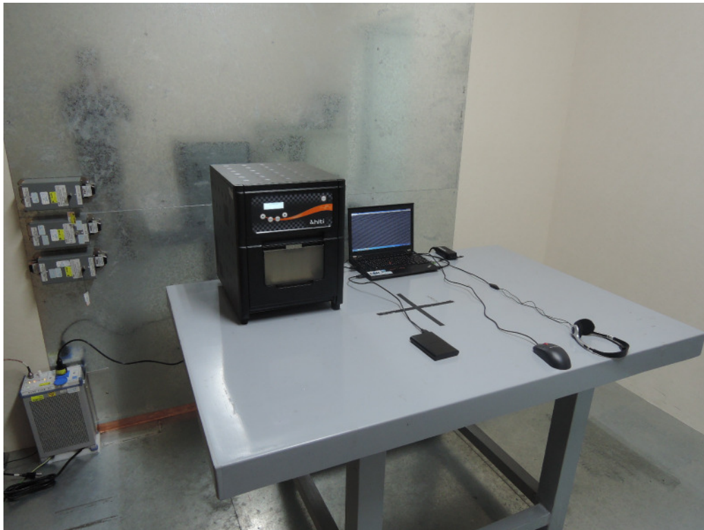
Photograph 5: Set-up for for Mains Conducted testing Back
