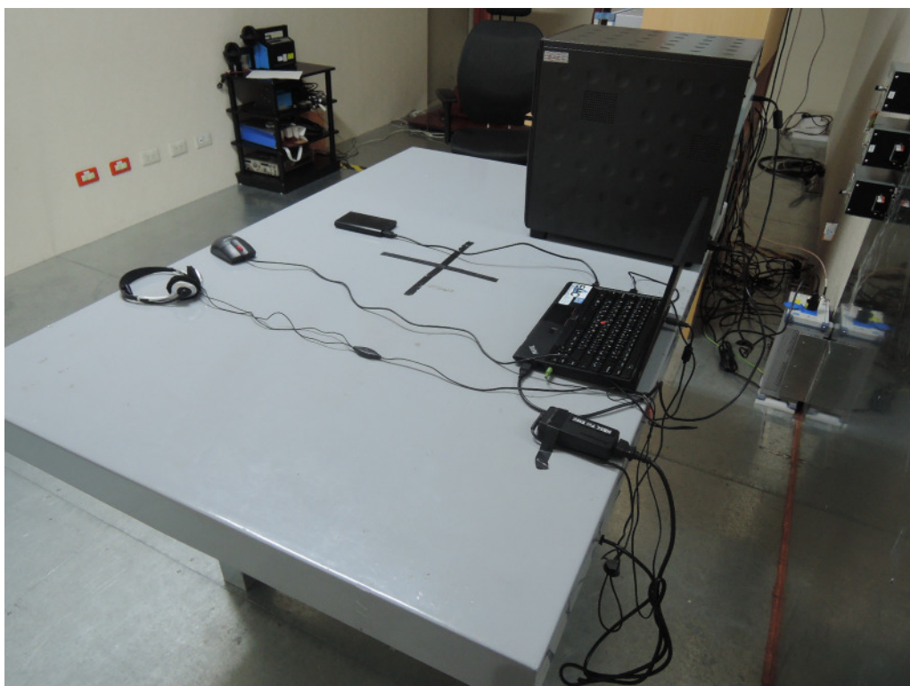
Photograph 6: Set-up for for Mains Conducted testing Front
