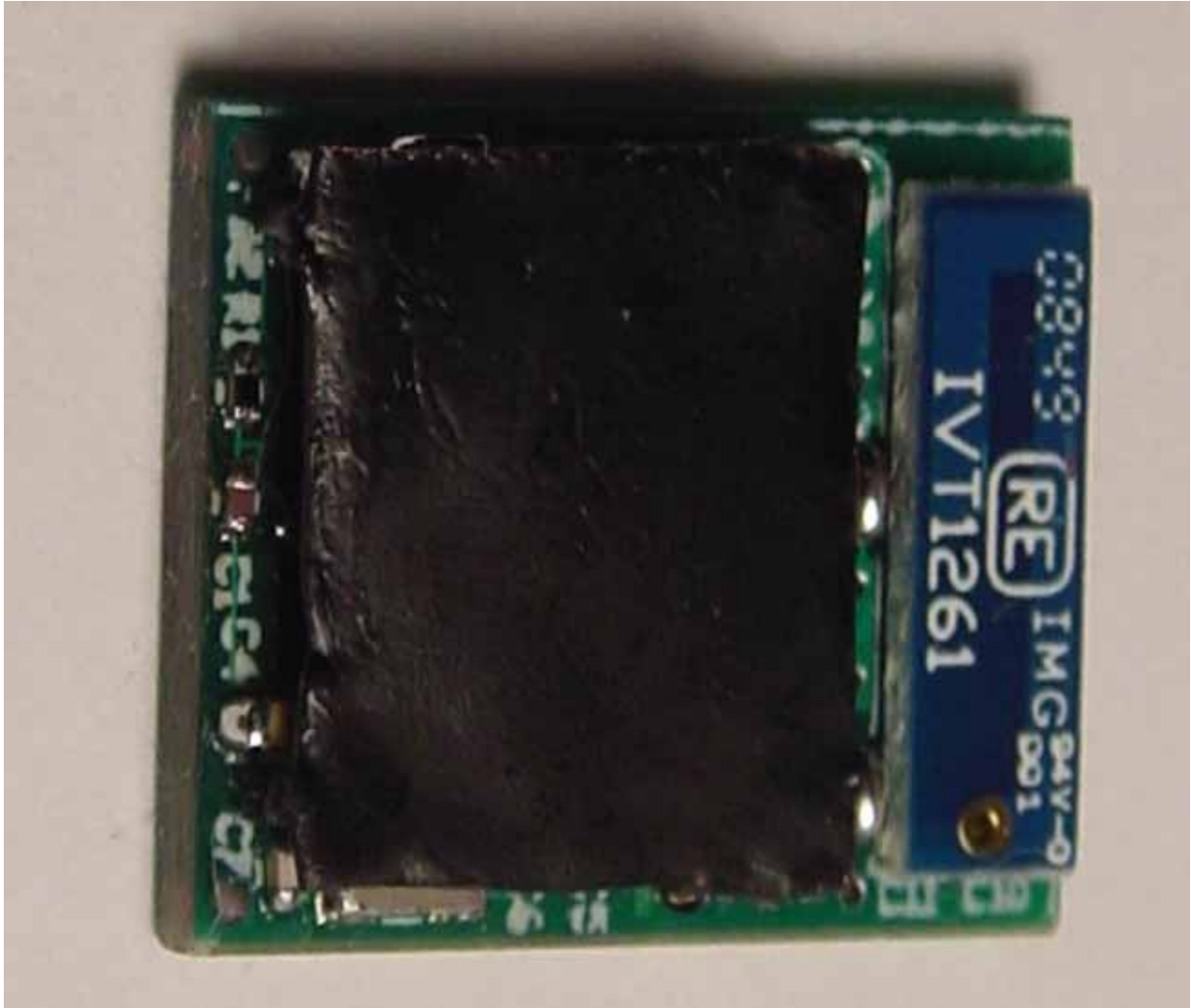
Photograph 8 - View of the Component Side of the EUT with RF Shield in Place
