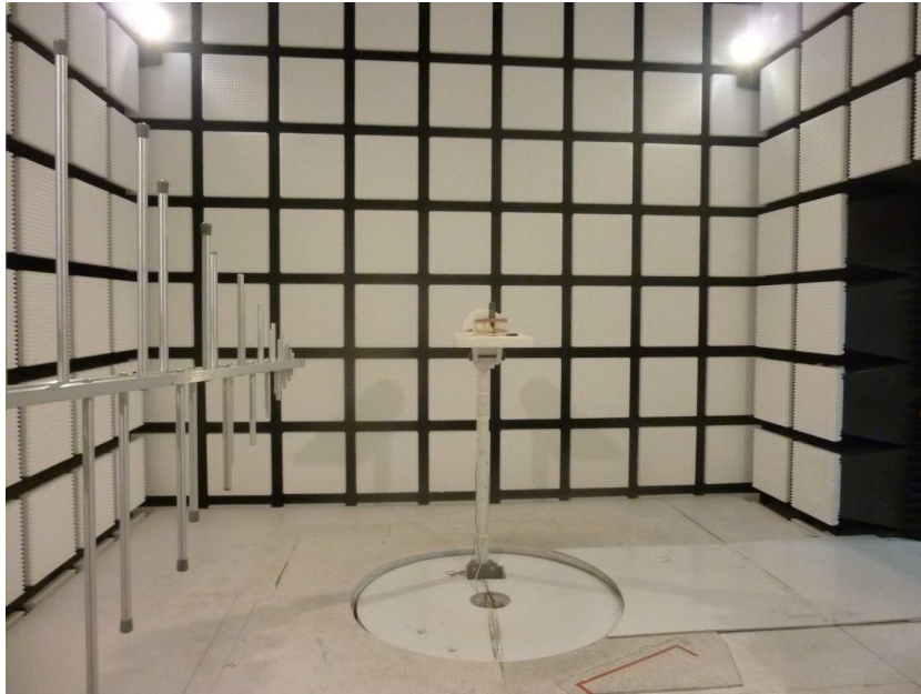
Photo 5: EUT at the anechoic chamber
