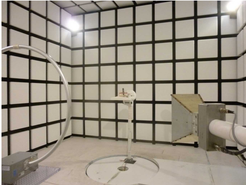
Photo 7: EUT at the anechoic chamber
