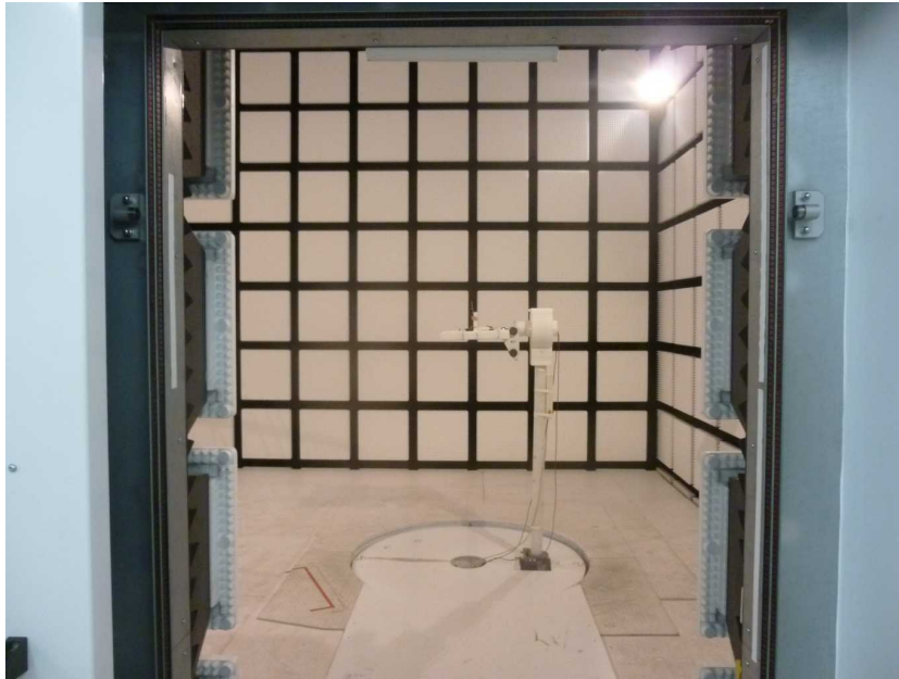
Photo 1: EUT at the anechoic chamber
