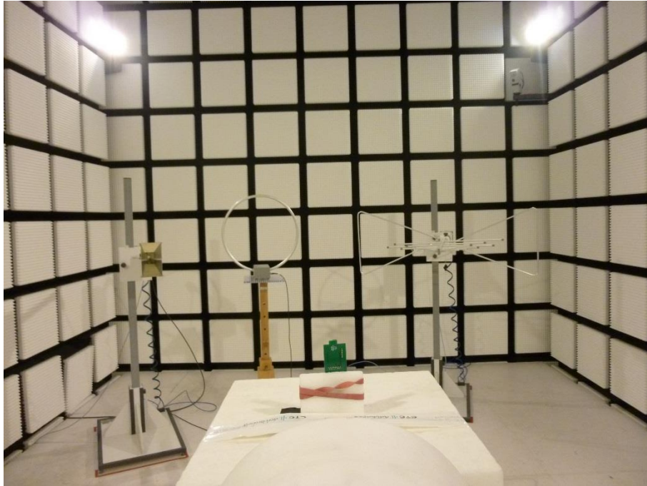
Photo 5: EUT at the anechoic chamber
