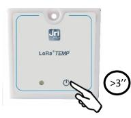
To activate the LoRa<sup>®</sup> *TEMP'* press and hold the On/Off button for more than 3 seconds. Once the device has been activated it starts measuring and transmitting data to MySirius at the set intervals.
