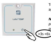
To turn off the LoRa<sup>®</sup> *TEMP'*, press and hold the On/Off button for approximately 3 to 6 seconds.
