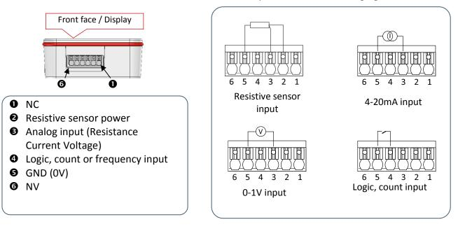
/!\ Connect only sensors which are compatible with the technical characteristics of the devices Sensor default detection is not possible in 0-20mA and 0-1V.
