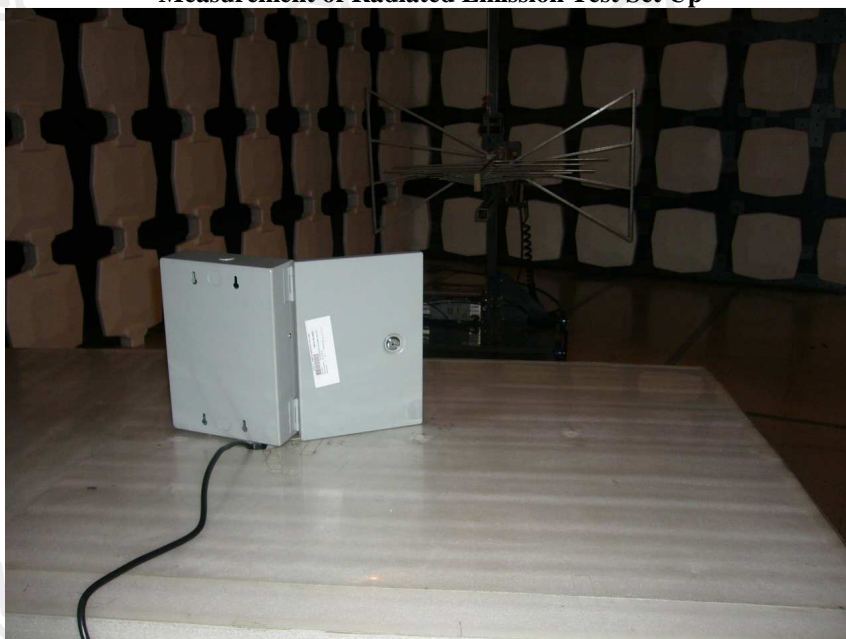
Measurement of Radiated Emission Test Set Up
