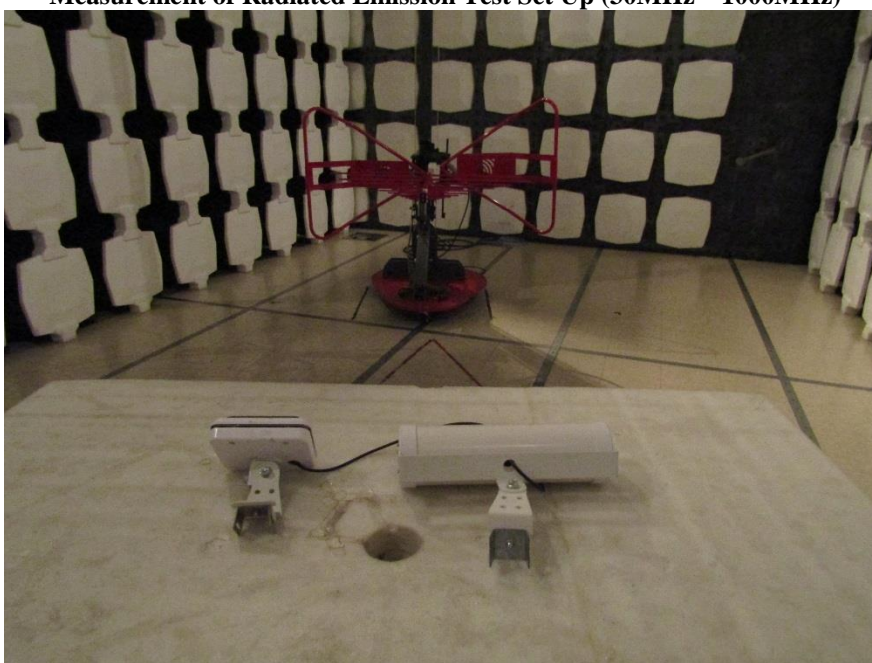
Measurement of Radiated Emission Test Set Up (30MHz – 1000MHz)
