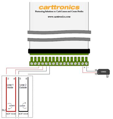
Fig.4 Sentry Connection Diagram
