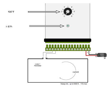
Fig.2 TX2 Connection Diagram
