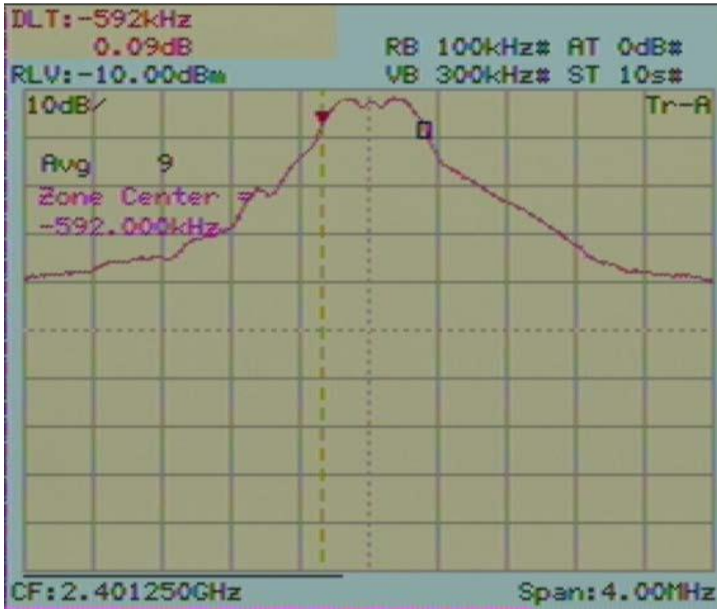
Figure 2 – Program Download mode emission mask
