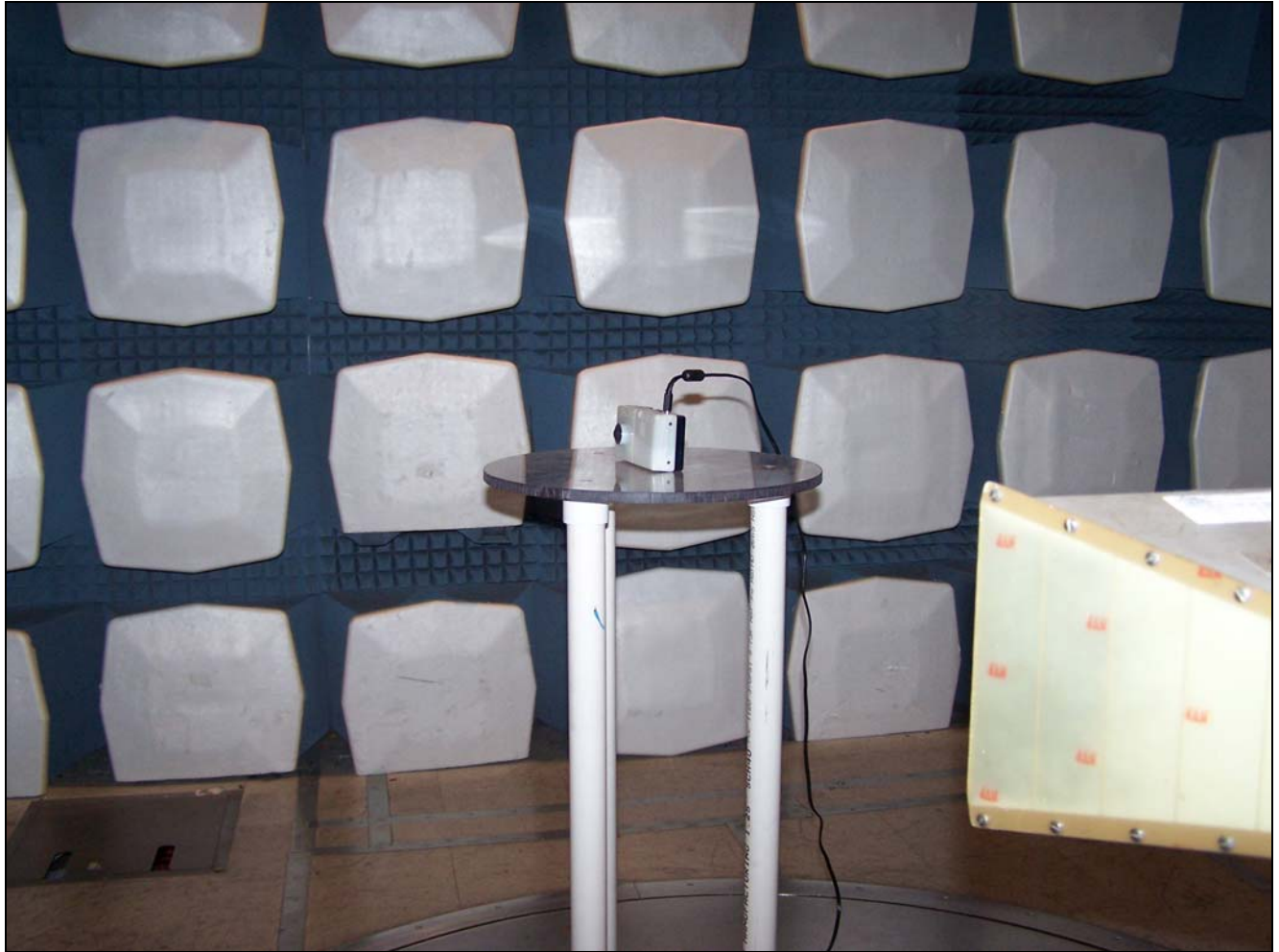
Photograph 3. Radiated Spurious Emission and Radiated Band Edge, Test Setup
