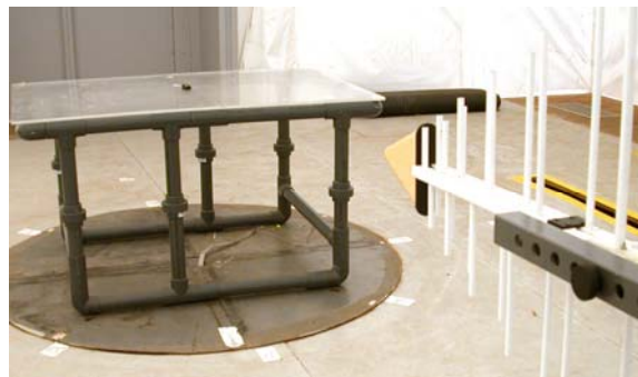
Figure 2-2 Radiated Emissions Test Set-up
