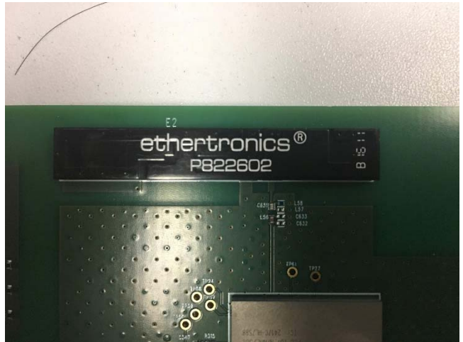
Antenna View - Cellular
