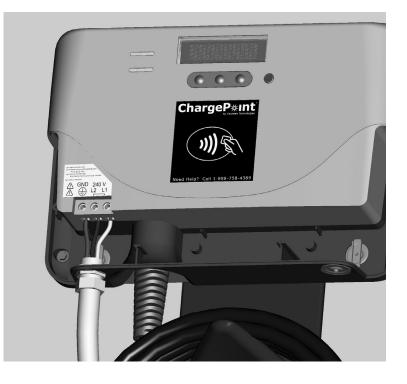
Use copper conductors only. Input terminal recommended tightening torque: 18.5 in.-Ibs. (2.1 Nm) Input terminal wire size range: 6 to 10 AWG (13mm<sup>2</sup> to 4mm<sup>2</sup>) solid / stranded.
