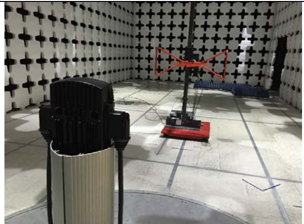
Radiated Emissions (<1GHz) - Rear View
