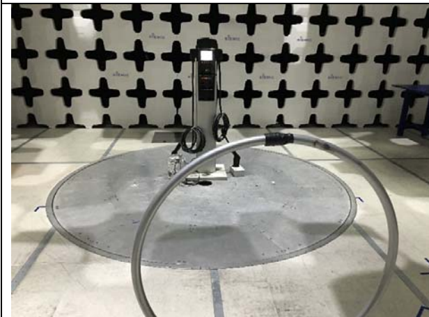
Radiated Emissions (<30MHz) - Front View
