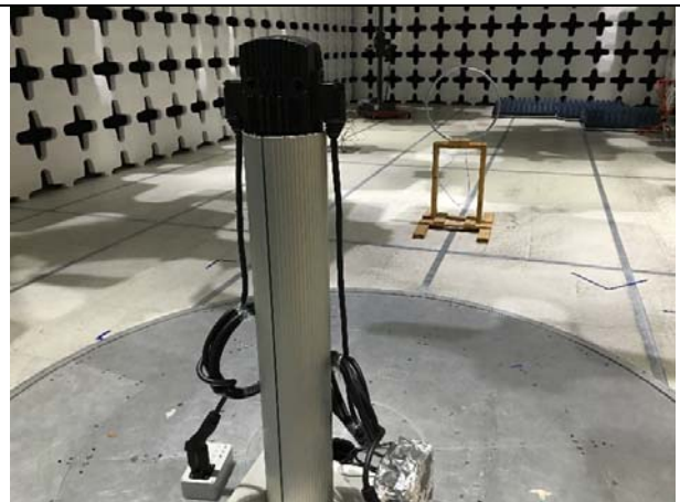
Radiated Emissions (<30MHz) - Rear View
