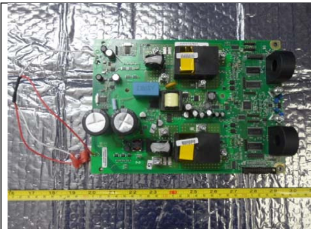
PCBA – Power Supply Top View
