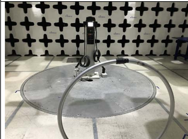
Radiated Emissions (<30MHz) – Front View
