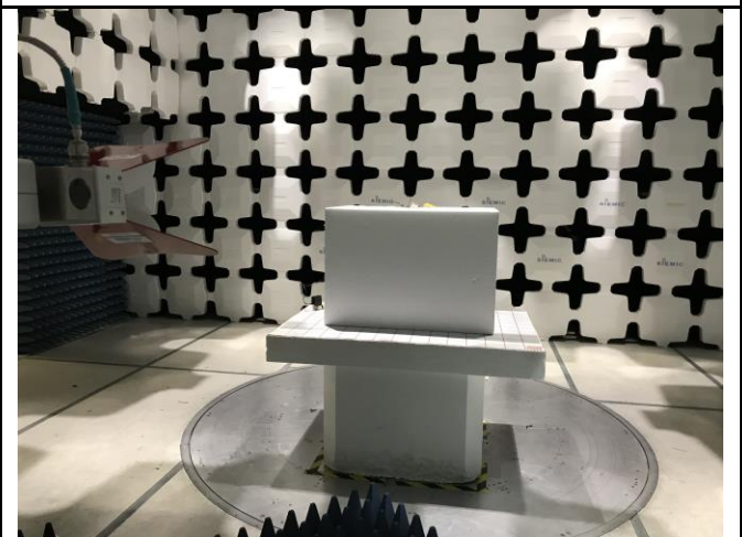
Radiated Emission Above 1G – Rear View
