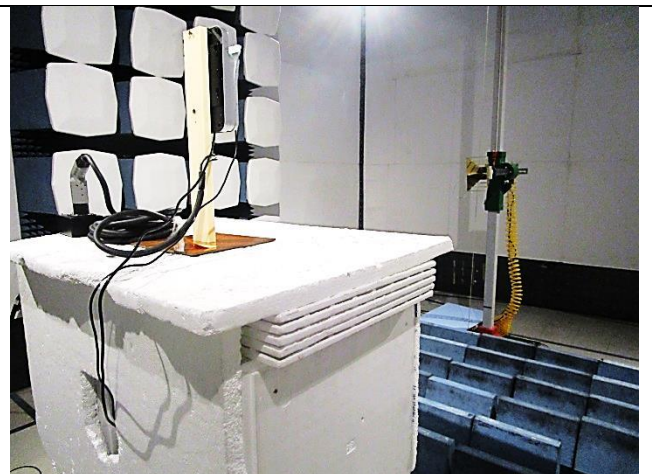
Radiated Emissions (>1GHz) – Rear View
