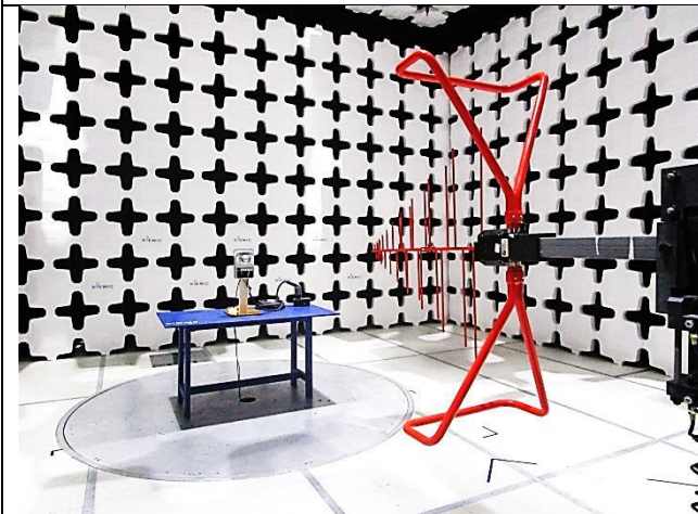
Radiated Emissions (<1GHz) – Front View
