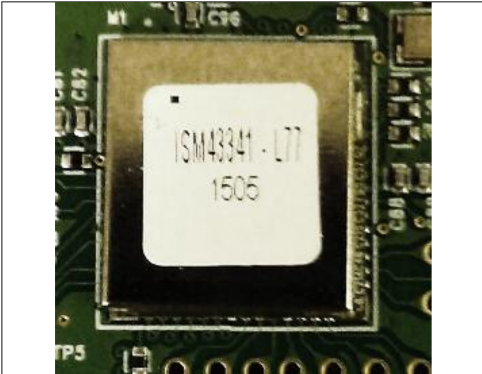
EUT Radio with shielding
