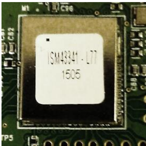
EUT Radio with shielding
