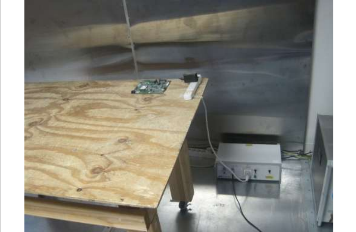
Conducted Emission Test Setup – Front View
