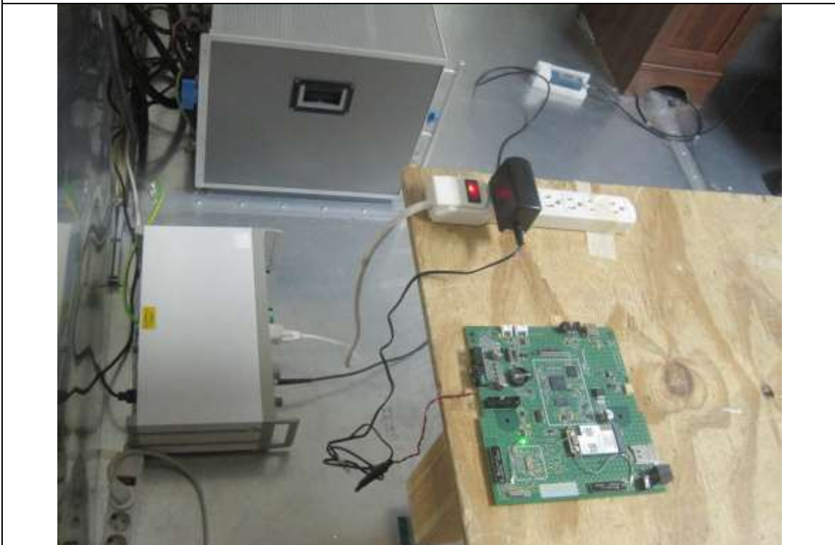
Conducted Emission Test Setup – Rear View
