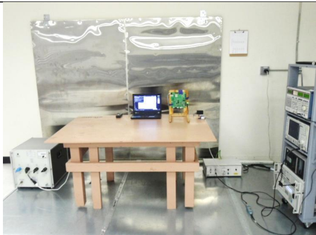
Conducted Emissions – AC Line Front View
