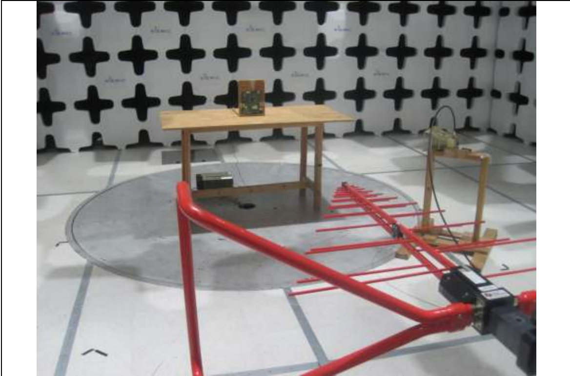
Radiated Emission Test Setup (30MHz – 1GHz) - Front View
