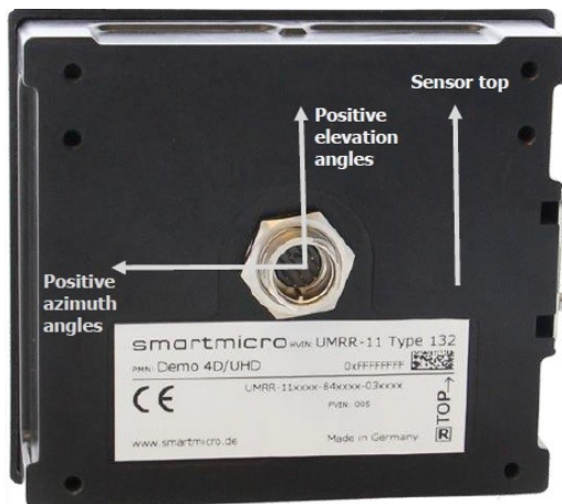
Figure 8: UMRR-11 Type 132 coordinate system (view from the rear side in the positive x-axis direction)
