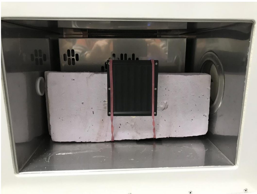
Photograph 6: Close View, without thermo shield (measurements were made only with thermo shield), T_{\min-\max}/V_{\min-\max}
