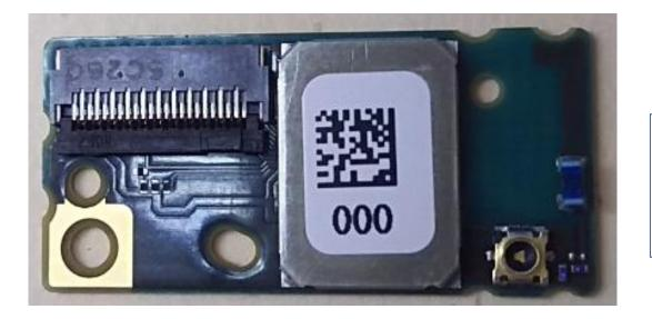
This connector is used for inspection only.
