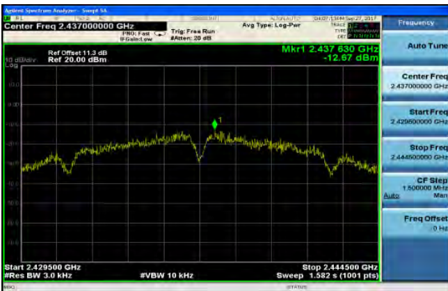
Power Spectral Density Test Plot (CH-High)
