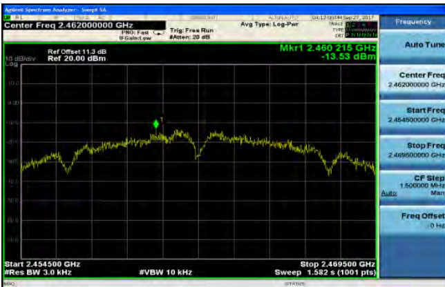
Power Spectral Density Test Plot (CH-High)
