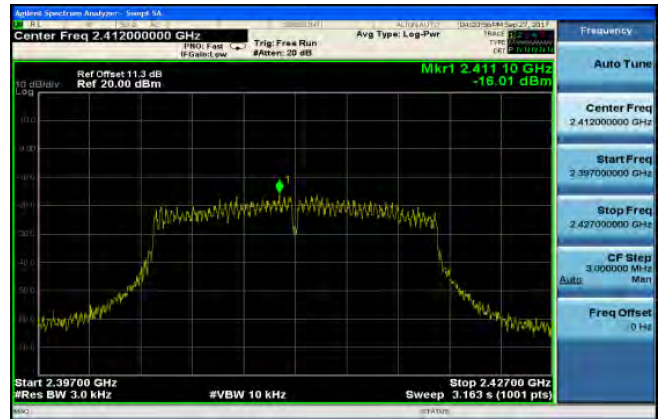
Power Spectral Density Test Plot (CH-Mid)
