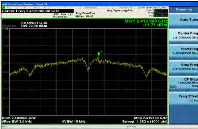
Power Spectral Density Test Plot (CH-Mid)
